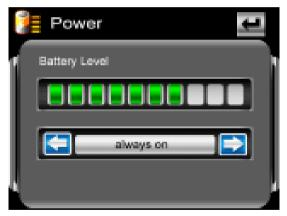
2, The "battery level "bar shows the current battery power and you can set the time to shut down automatically by clicking the two icons
